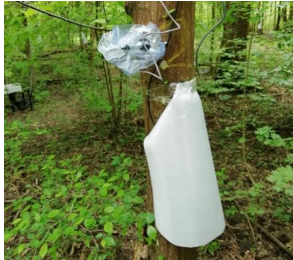
Photo: Sartori (2021). Note: the plastic bag is used to prevent moisture damage
