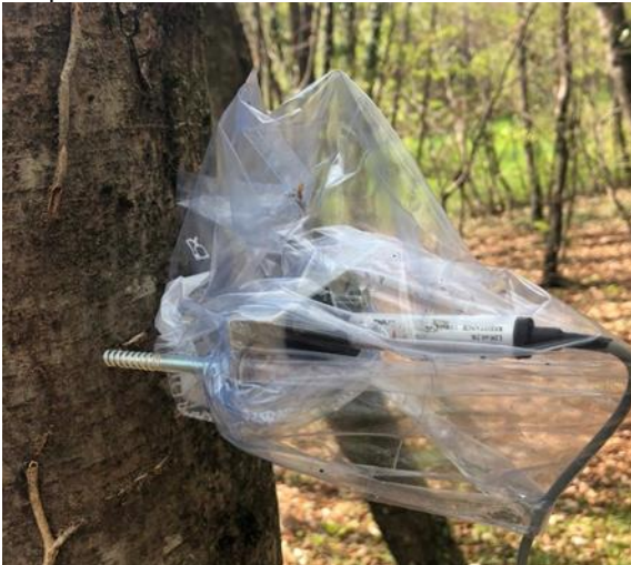
Photo: Vidale (2021). Note: the plastic bag is used to prevent moisture damage
